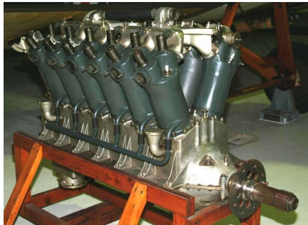
Liberty. Water-cooled V-12, used in many WWI airplanes, post-WWI airplanes, boats, and even some tanks. 420 hp at 1700 rpm.
