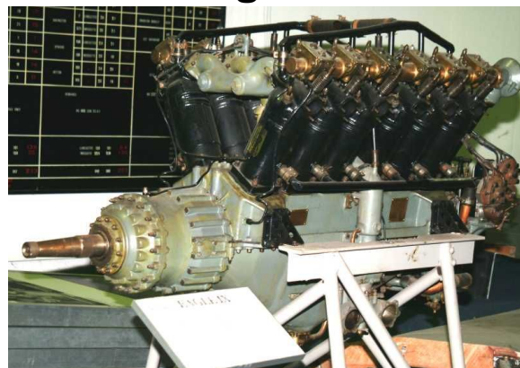
Rolls-Royce Eagle, 225 hp – 360 hp. Used in Handley Page O/400 bomber, Vickers Vimy bomber.
